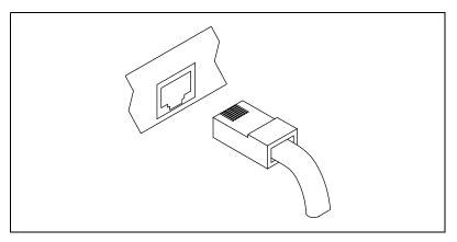
Figure 1. Connecting the Network Cable
